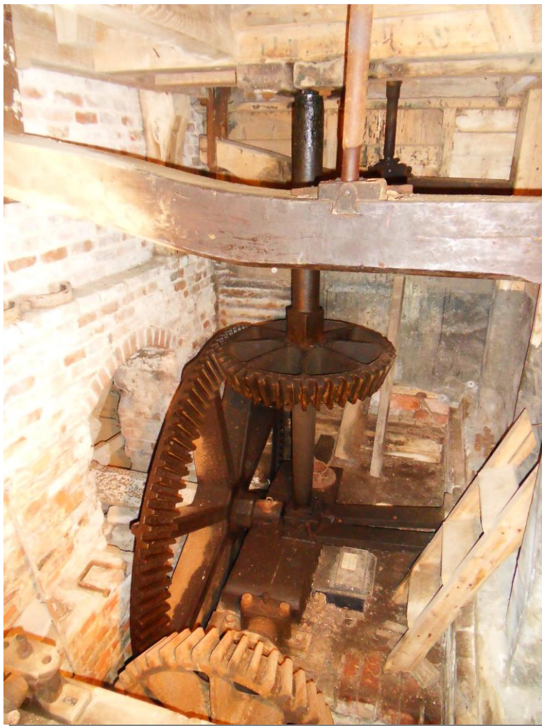
Fig.12 The iron Pit Wheel, bevel Wallower with ancillary power drive in the foreground; wooden Bridge Trees and millstone spindle above
